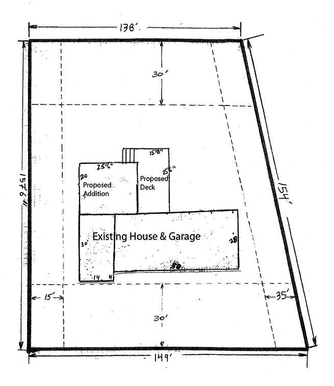
Sample of Plot Plan showing Existing Structure and Additions—required for all exterior alterations or new construction
